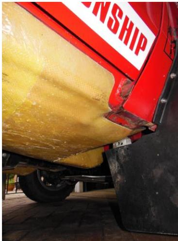
**Photo 1 caption:** Under arduous rally racing conditions the GMS EP-620 aramid fibre composite protector covers lasted twice as long as the original composite covers.
