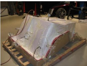
Caption for photo 1: The carbon fibre epoxy composite monocoque cockpit chassis was ‘out of autoclave’ moulded under vacuum from GMS EP270 epoxy prepreg at only 70 Deg C.
