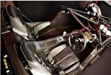
Caption for photo 3: This unique epoxy carbon fibre composite monocoque cockpit chassis, the first ever built in Australia is approximately 2 meters by 1.5 meters. It has all the torsional rigidity needed for this 6.0 litre V8 powered roadster sports car, yet weighs only 80 kg.
