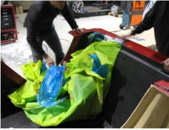
Caption for photo 2: For this one-off concept car, GMS EP270 epoxy prepreg provided the FR-1 design team with light weight and high mechanical performance, combined with being able to use cost efficient fibreglass tooling and a low temperature, low cost production process.
