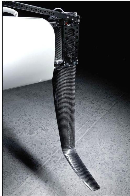
Photo 2 caption: The higher mechanical performance of the GMS Composites epoxy carbon laminate system combined with the proprietary design and shape of Paradox foils enables a single dagger foil to support the full weight of the boat plus the dynamic loads when racing at high speed.
