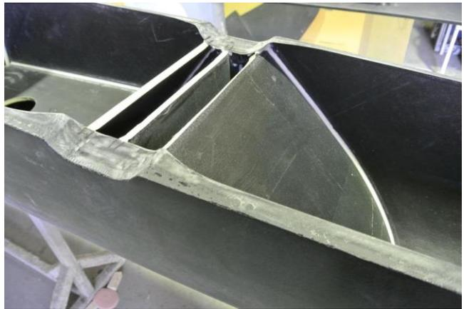
**Photo 2 (a), (b), (c) and (d) caption:** Using a customised GMS EP-270 epoxy prepreg with an S-glass cloth multilayer combination, provided Windrush Yachts with the best high performance dynamic strength properties, and thinnest, lowest weight, GRP outer laminate possible for its Tornado catamaran honeycomb sandwich composite hull design, according to ISAF build design restrictions.
