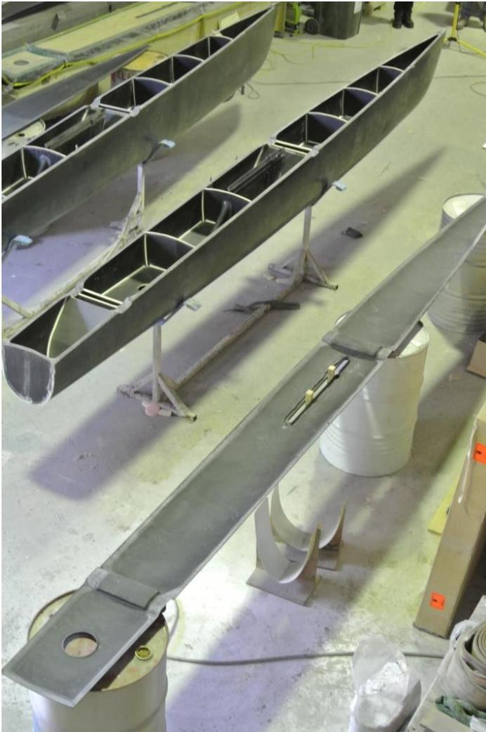
**Photo 3 caption:** The ‘carbon free’ epoxy based composite hull and deck structure needs to be stiff enough to take the immense sail rig forces, yet still provide the high speed ‘slam’ impact resistance and flexural bending demands placed on a single hull when racing.
